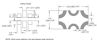
NOTE: When wave soldering, the gap between pads should be covered with photo-imageable solder mask to prevent bridging between terminations under the component. Also the spacing between the ground contacts should be increased from .635mm (.025") to .889 (.035").
